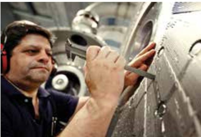
A mechanical maintenance supervisor checks the groove depth of a Finebar® plate. The original OEM plates at Setúbal were a 48" diameter with a cutting edge length (CEL) of 167 km/rev. These large diameter patterns consumed no load power of 240 kW.
